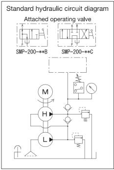
⚠ When the pump is used continuously, caution should be paid to rated operation time and the increase in the motor and oil temperatures.
