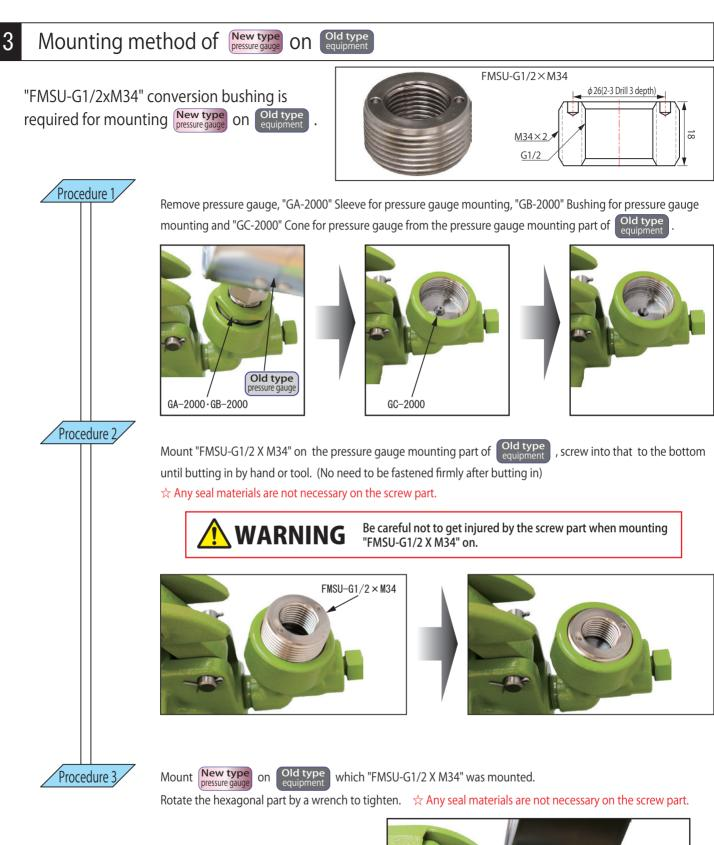
Tightening torque 39-59 N•m
